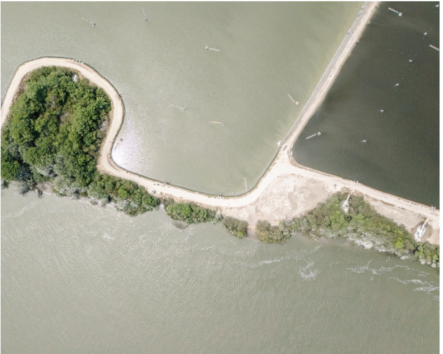
Mangroves partially cover a dyke separating shrimp farm ponds from a large canal. Water from one of the ponds drains through pipes into the canal.
